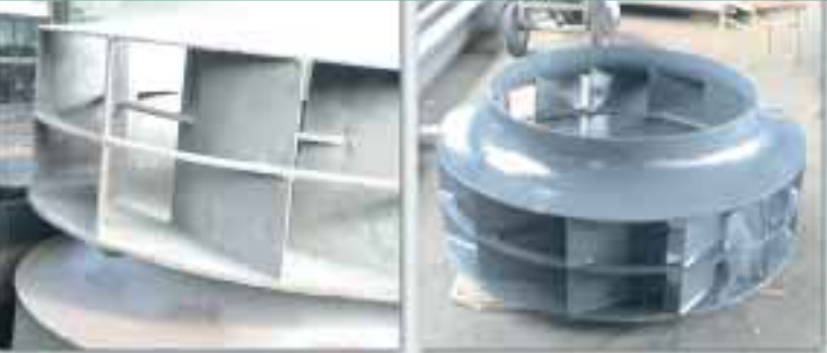
Two impellers before abrasive blasting
