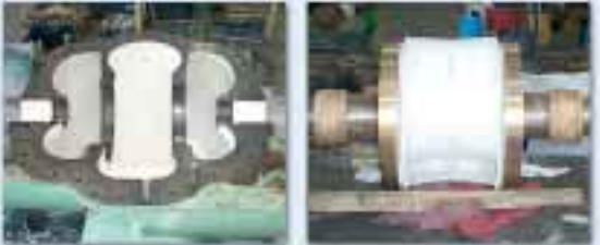
Repair the worn and corroded shaft using Loctite® 3478 Superior Metal. After it's cured, machine it to complete the repair. Coat all parts with Loctite® Nordbak® 7228 Brushable Ceramic White (certified for use in contact with drinking water).
