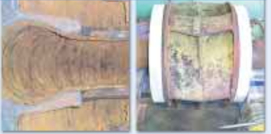
Top cap and bronze impeller before repair. The first step is to abrasive blast these parts to SA-3 White Blast 75 µm profile.
